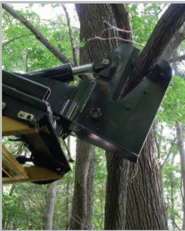
Head rotates 90° to vertical position allowing for the cutting and pruning of limbs and bows.
