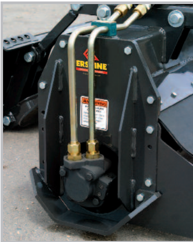
Hydraulic motor mounts inside the exclusive Direct Drive Rotor eliminating reduction chains, sprockets, gears, or bearings.
