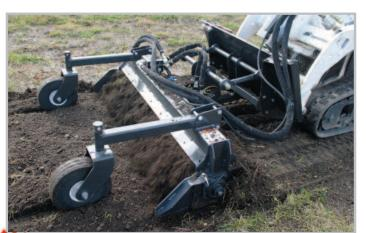
ordinary tiller, with the benefit of faster ground speed. The counterrotating rotor moves soil ahead of it as it tills, filling in low spots and chewing off high spots. It creates perfect seedbeds and windrows. This attachment separates rocks, tears up sod, and pulverizes dirt clods. It rakes and tills as deep as 2".
